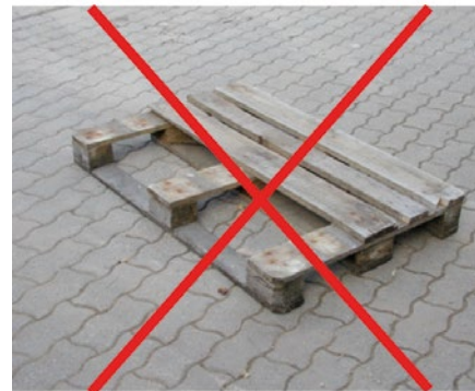
Splintered top edge board
